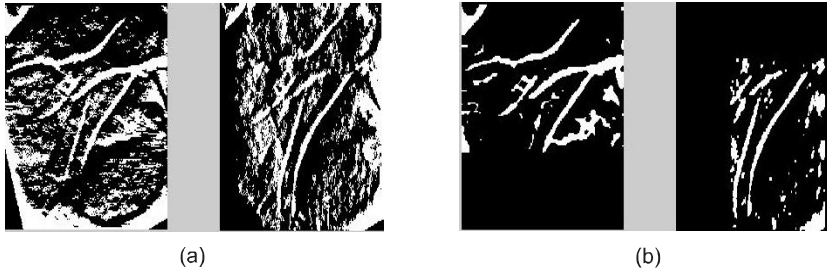
Figure 5. (a) Horizontal ( I_{g-x} ) and Vertical edges ( I_{g-y} ), (b) Filtered horizontal ( I'_{g-x} ), and Vertical edges ( I'_{g-y} ).
